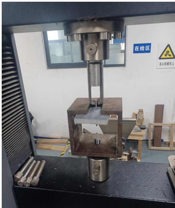
Direct Screw Withdrawal Test (Screws driven into fiber cement board only)
