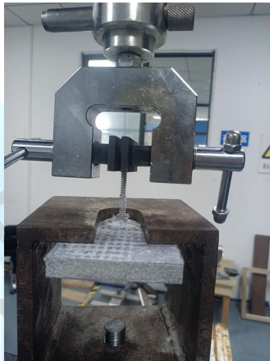
Screw-Head Pull Through Test (Screws driven into fiber cement board only)
