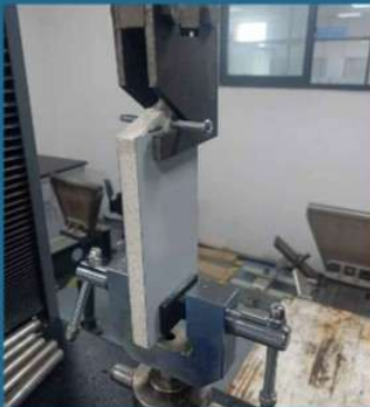
Screw lateral resistance test
