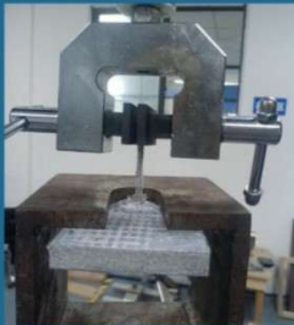
Direct screw withdrawal test
